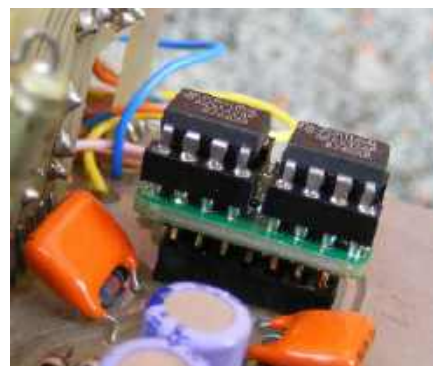
Rysunek 4. Adapter two-duals-to-quad zainstalowany w starym mikserze Audio Developments
