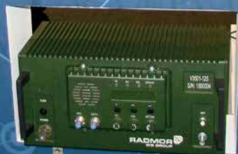
V3501 vehicular radiostation
