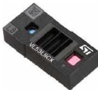
Fotografia 13. 64-polowy sensor dToF marki ST Microelectronics ( https://t.ly/2SjtH )
