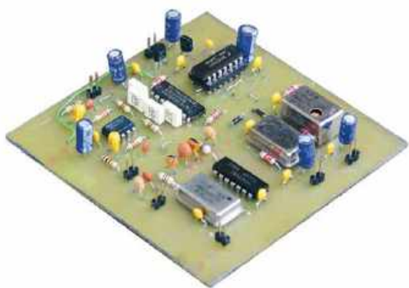
Odbiornik SDR kit AVT2934 wg SQ4AVS
